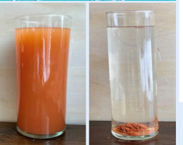
Silt Clear<sup>™</sup> powders are high quality anionic polyacrylamide blends designed specifically for turbidity removal in passive water treatment. With dual benefits of water clarification and soil stabilization. Silt Clear™ can transform traditional sediment control BMPs into water treatment devices capable of removing upwards of 90% of fine silt, clays, metals and nutrients.
