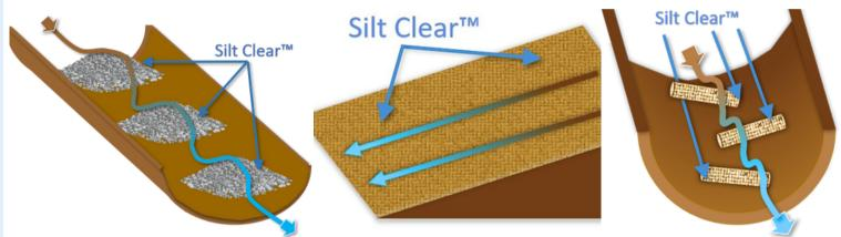
Silt Clear™ can be applied to rock checks (left), matted slopes (middle), wattles (right) and many other existing BMPs!
